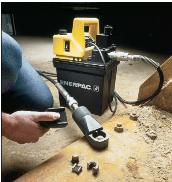
◀ This PED-1001B Submerged pump quickly and quietly powers a hydraulic nut cutter in this bucket maintenance application.
