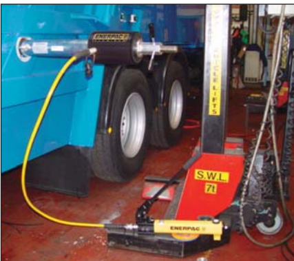
◀ An RACH-306, powered by a P-392 hand pump, is used to extract corroded carriage pins from refuse collection vehicles.
