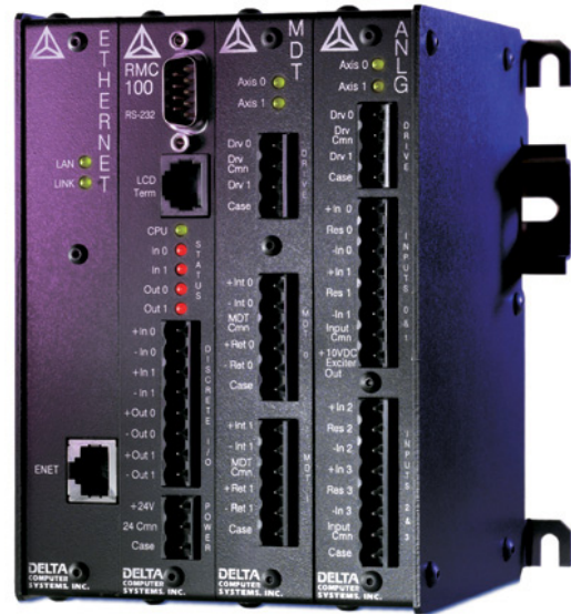
Figure 2. – A well-connected motion controller provides direct interfaces to transducers as well as system buses. This is the RMC100 from Delta Computer Systems, Inc.
